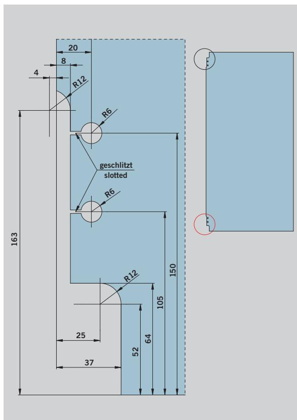
Drawing shows the bottom glass penetration. Top edge of glass is prepared accordingly.
