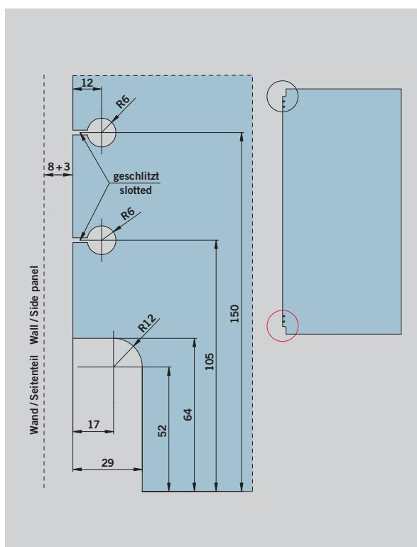
Drawing shows the bottom glass penetration. Top edge of glass is prepared accordingly.
