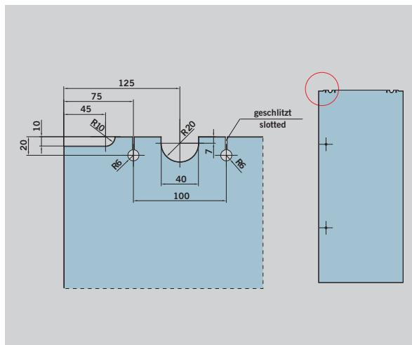
Irrespective of the door width, the glass preparation (LH edge shown here) applies correspondingly in mirror image for the right edge.
