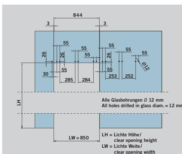
for a toughened glass assembly, clear opening width 850 mm.
