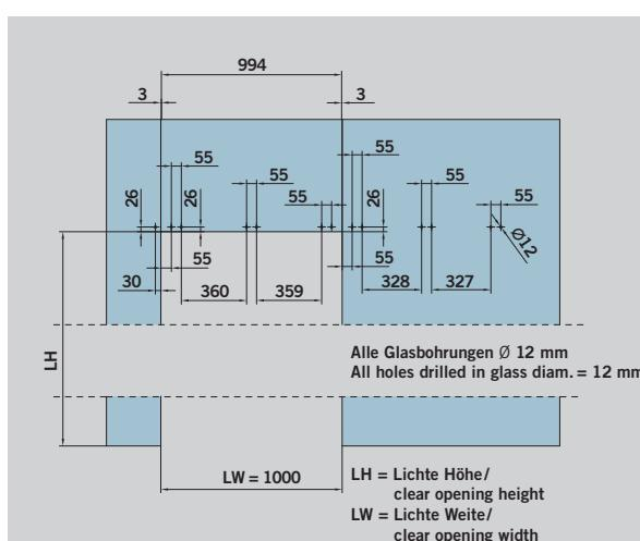
for a toughened glass assembly, clear opening width 1000 mm.
